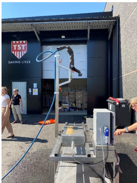
Figure 3 Cobra test lance fixed to the rack
