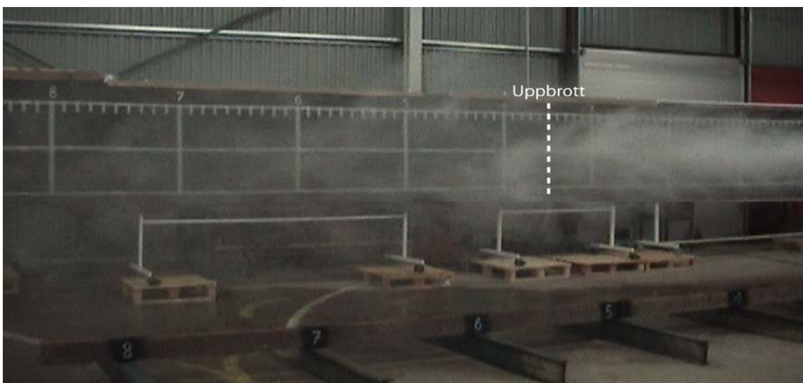
Picture 18 Water jet which breaks through a test body. ( Uppbrott = break up )
