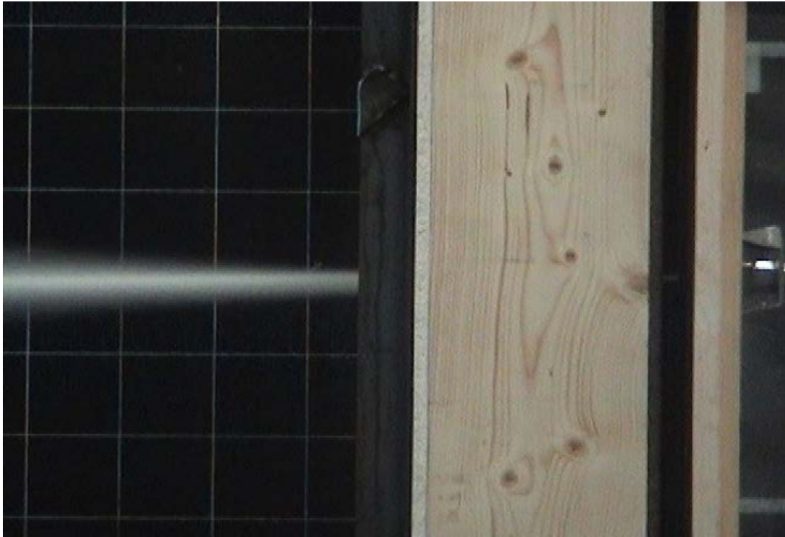
Picture 17 Impact of the water jet after penetration of the test body.
