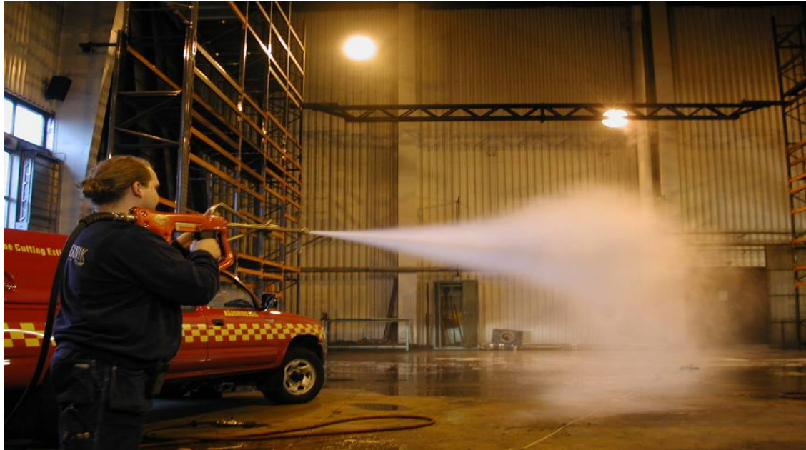
Picture 15 Trials with the cutting extinguisher lance to determine the influence of additives on the break up and throw length.
