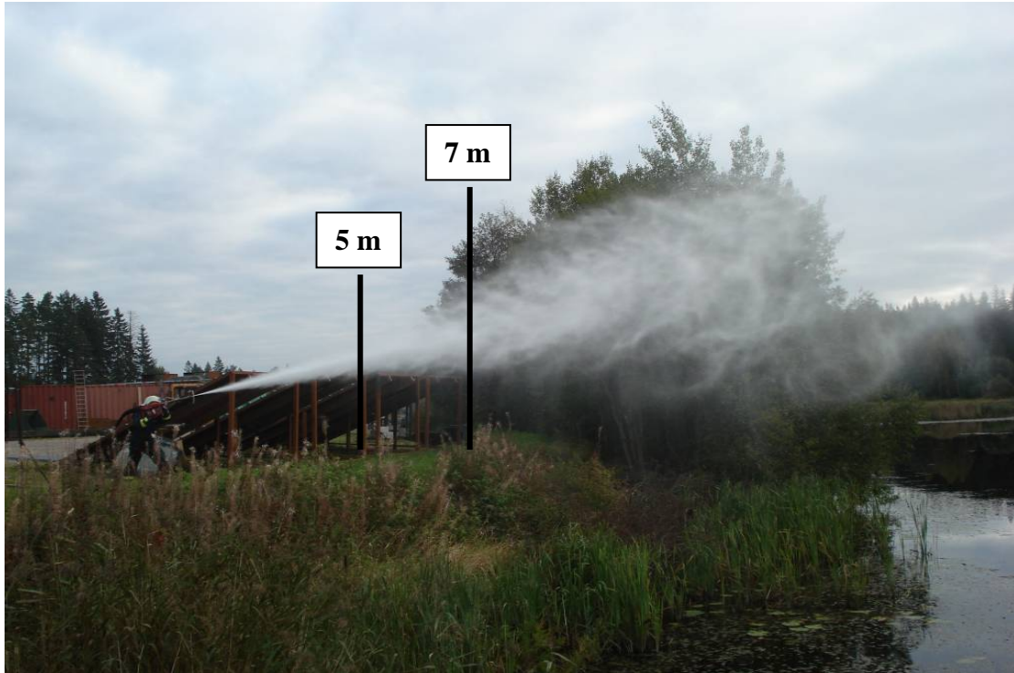
Picture 16 Demonstration experiments at the Guttasjön training area in Borås showing how the beam breaks up only after approximately 5 meters and is completely broken up after approximately 7 meters.
