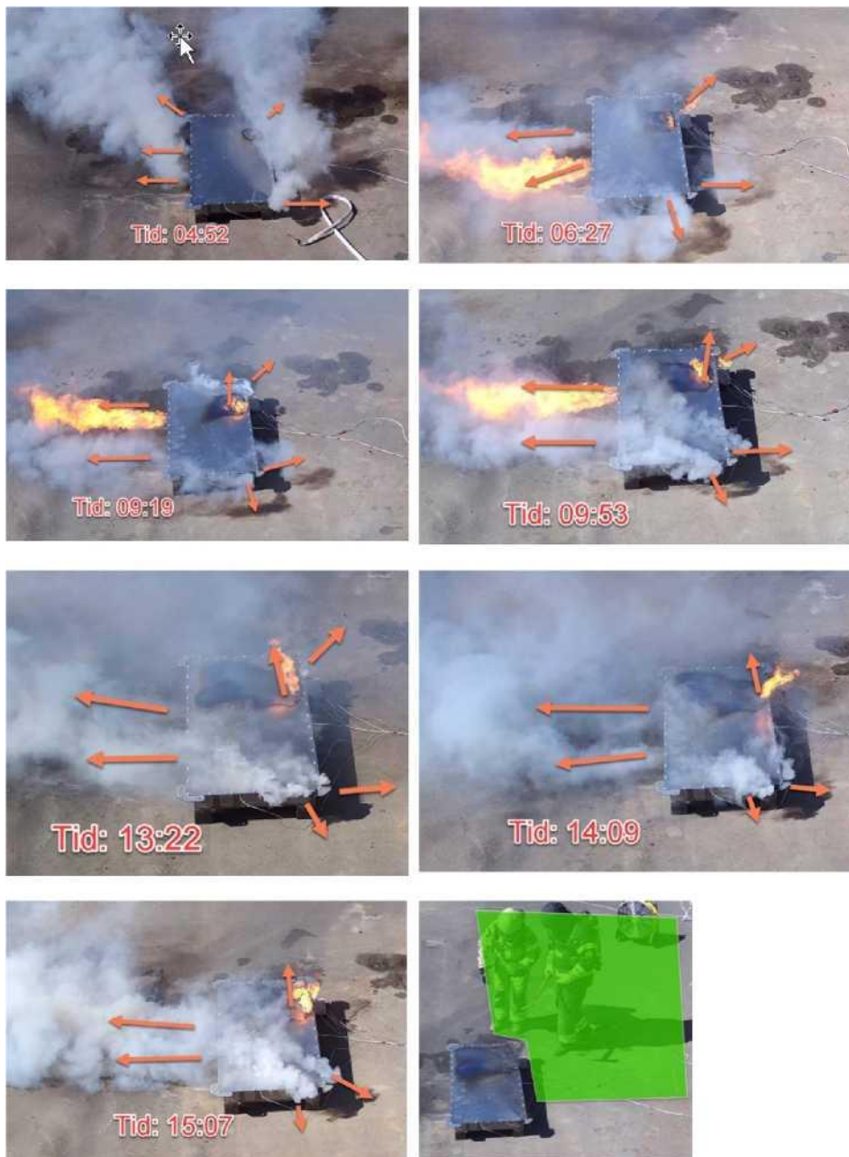
Figure 22. Example of smoke and flame propagation from the sub-pack in test 1C. The thermal propagation pattern varies between different vehicles and battery architectures and must be studied on a case-by-case basis before first responders approach the fire scene. The green shape shows the area deemed safe in this case.
