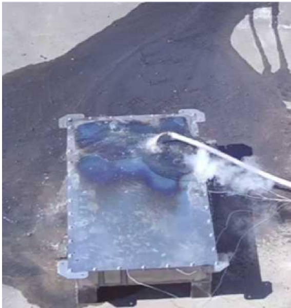
Figure 12. Firefighting with narrow hose and copper pipe - test 1C.
