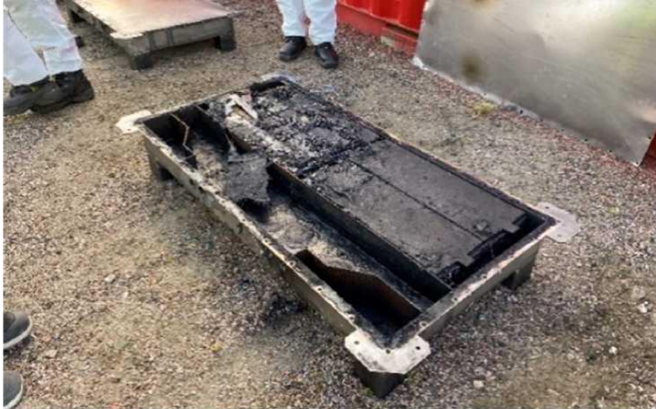
Figure 7. Sub-pack after extinguishing with a cutting extinguisher.
