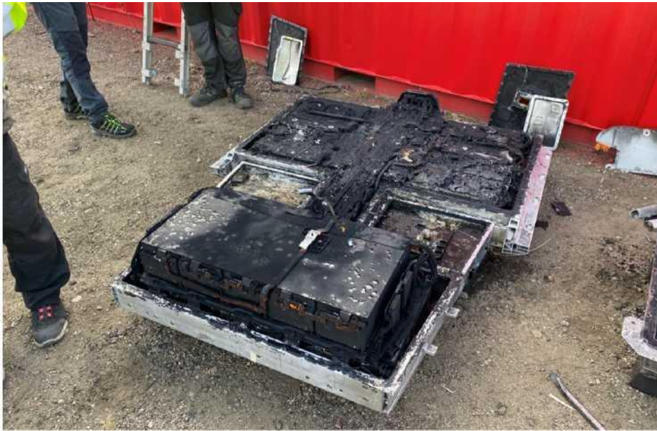
Figure 17. Detached electric car battery after extinguishing with lid removed - test 2.
