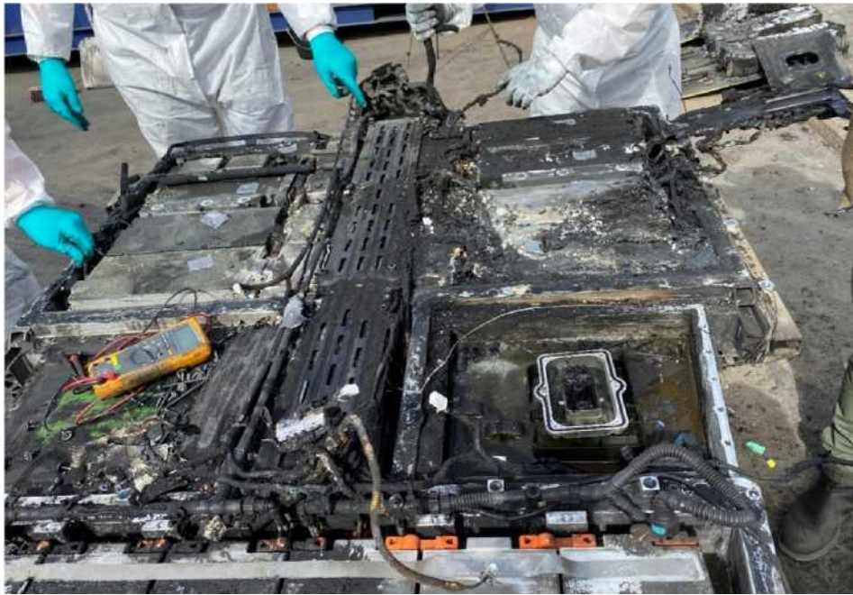
Figure 20. Battery pack removed from electric vehicle after extinguishing - test 3.
