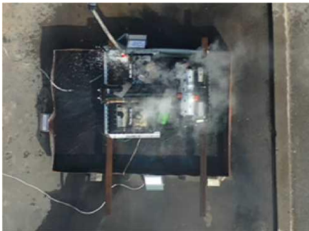
Figure 15. Extinguishing with narrow hose and spray pipe - test 2.
