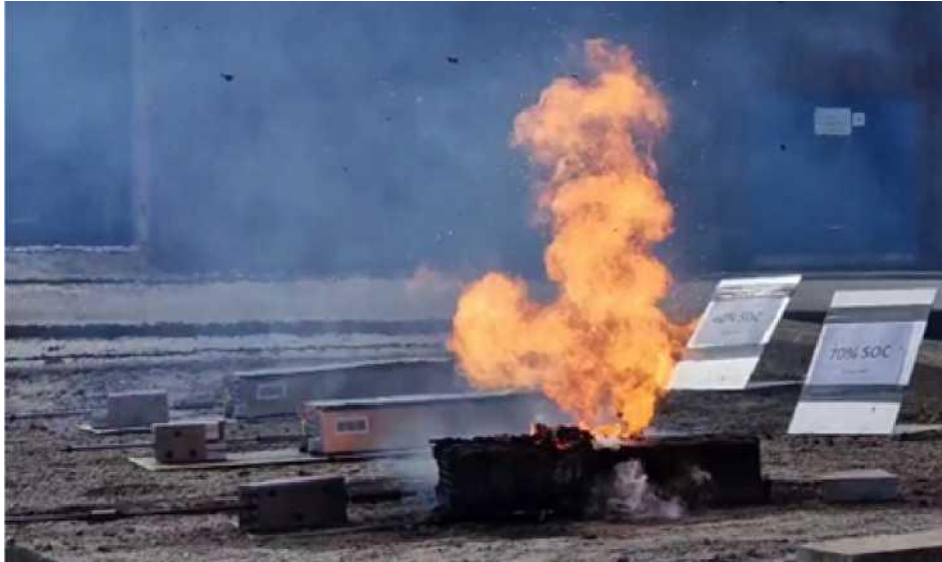
Figure 21. Course of fire in battery module (100 % SOC).
