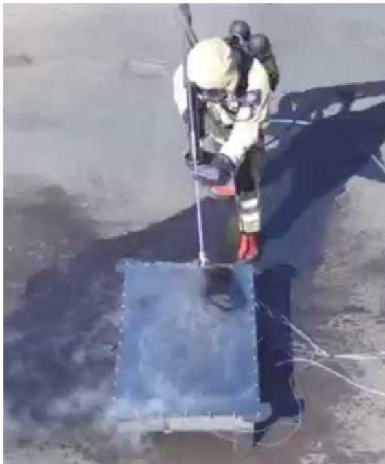
Figure 6. Firefighting with cutting extinguisher - test 1A.
